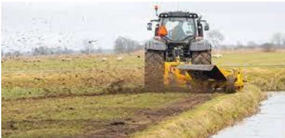
Figure 5: Spreading arisings left on bank top (Bos rotary cutter WA-150)
