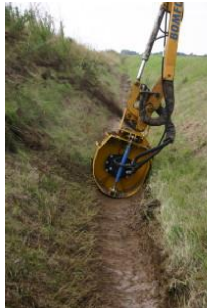
Figure 3: Desilting and spreading using a boom-mounted spreader (Klose Engineering)
